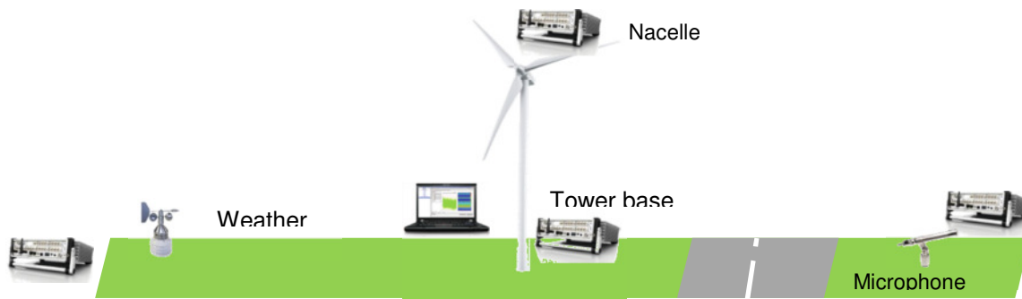
Figure 5: Exemplary wireless setup for a measurement campaign at a wind turbine
