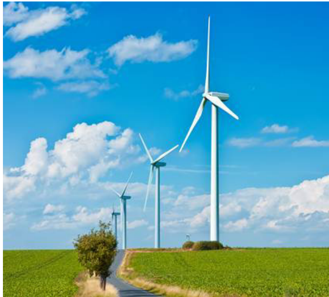
Figure 3: Exemplary influences on the measurement setup. The trees, the street and neighboring wind turbines influence the acoustic measurement
